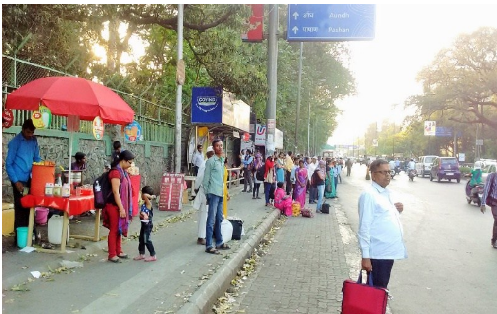
Figure 12: Ill-designed Bus stops creating blockage for pedestrian and cycle movement
