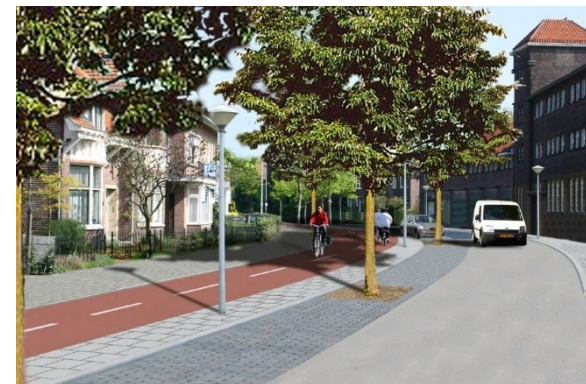
Figure 33: One-way, one lane road with two-way cycle track (this road used to have two traffic lanes)
