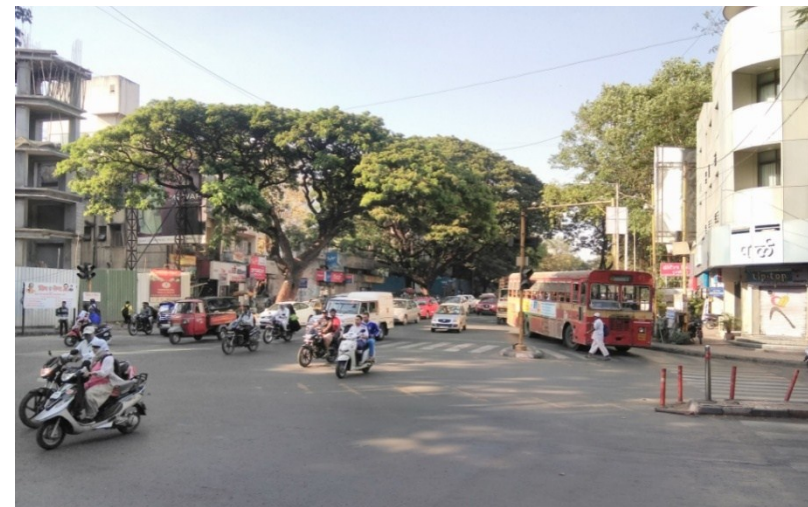
Figure 41: Lack of Road safety. Left-turn slip roads allow vehicles to keep their speed when turning left.
