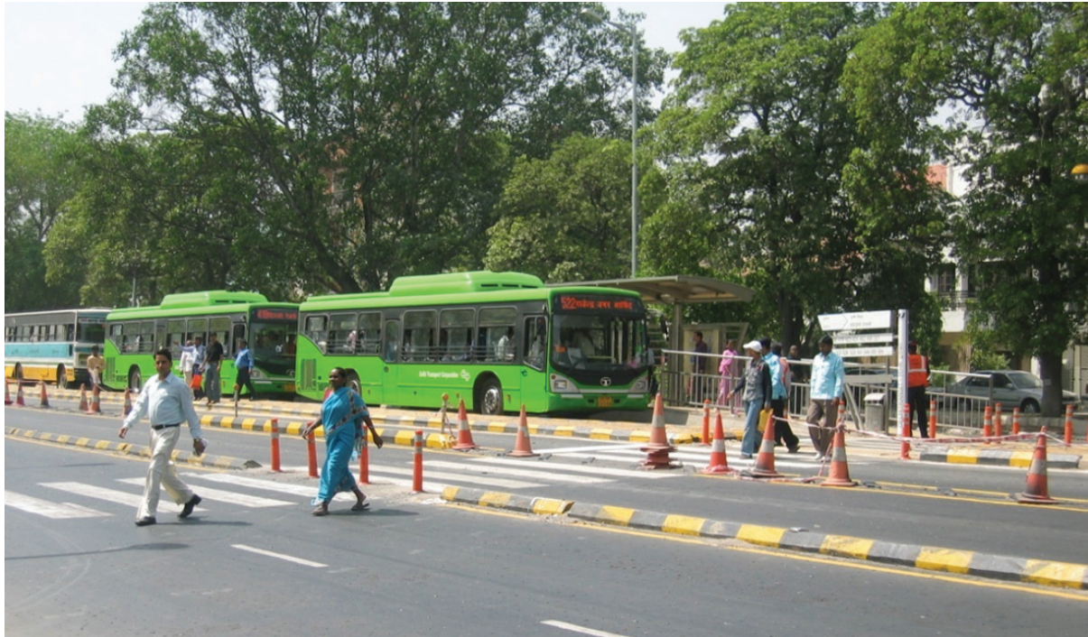
Figure 11: At-grade pedestrian crossing mid-block
