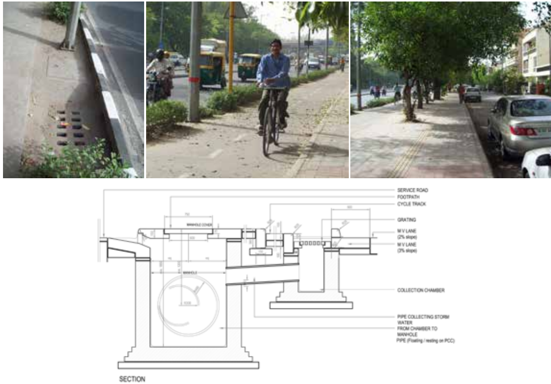
Figure 36 : Drainage for arterial streets (Source : SGArchitects, Delhi)
