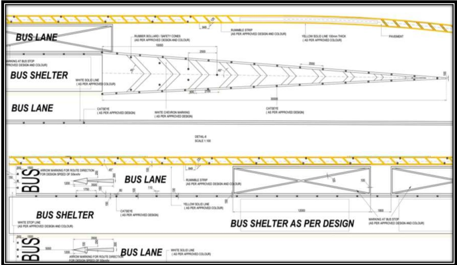
Figure 8-13 : Bus marking – along the carriageway
