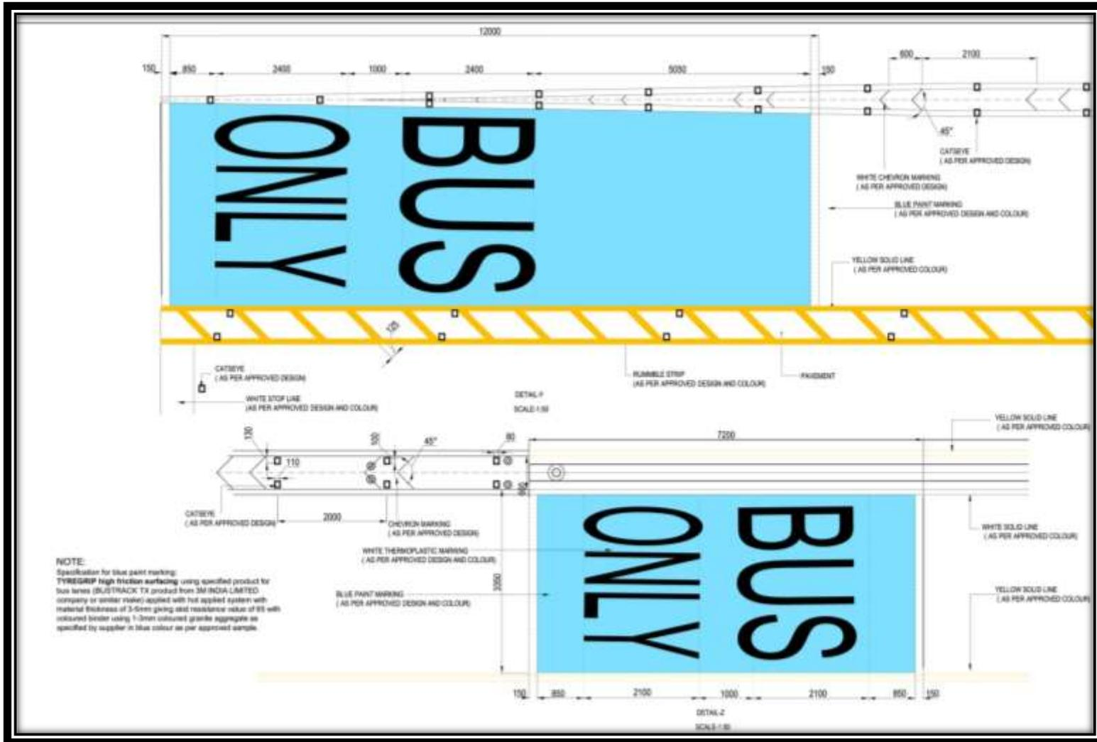
Figure 8-15 Typical marking at junctions for Buses
