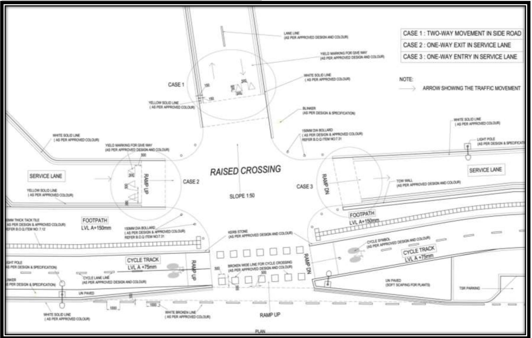
Figure 8-18 : Making at raised crossings
