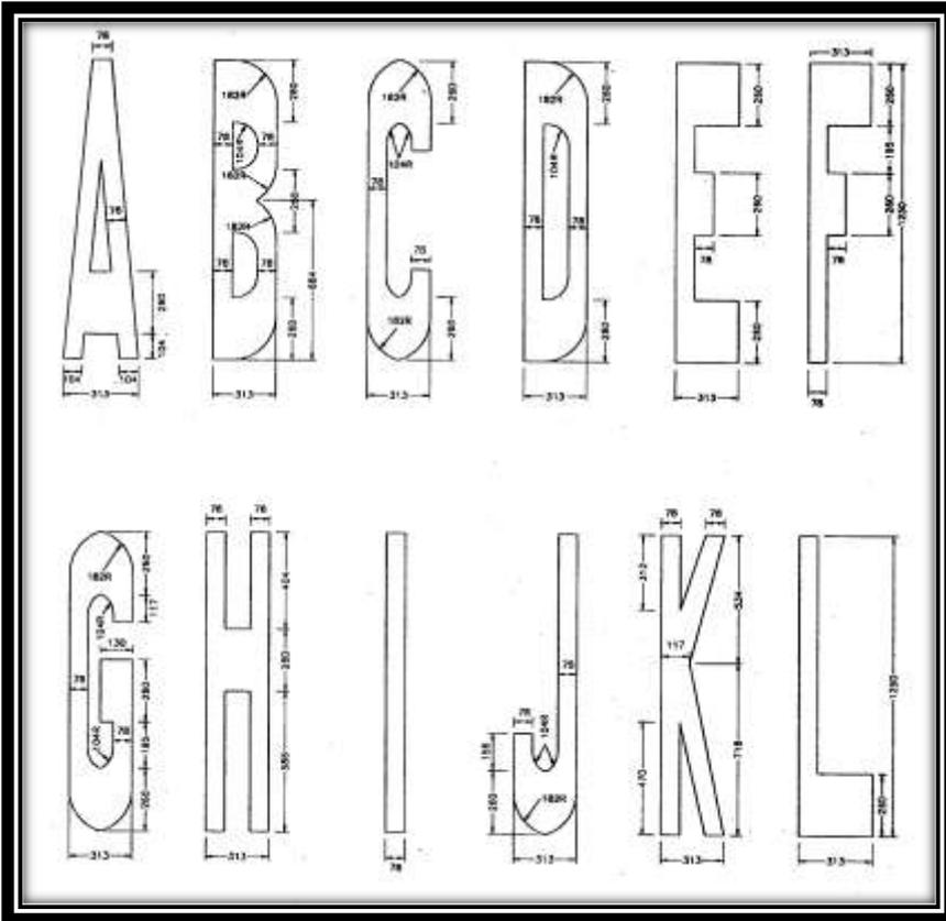
Figure 6-1 Size of the letters for word messages (speed 50 km/h or less)<sup>5</sup>
