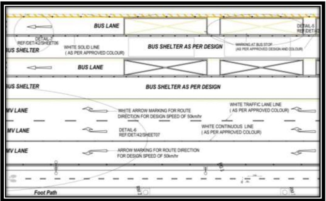
Figure 8-1 : Typical marking before the junction for all road users
