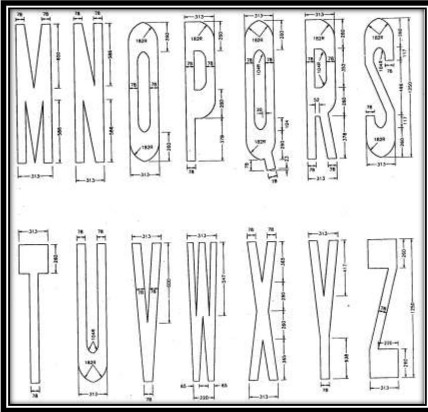
Figure 6-2 Size of the letters for word messages (speed 50 km/h or less)<sup>6</sup>
