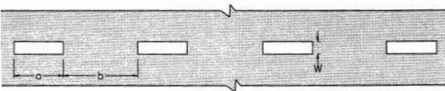
Figure 8-2 - Centre line where a and b depends upon the no. of lanes of carriageway
