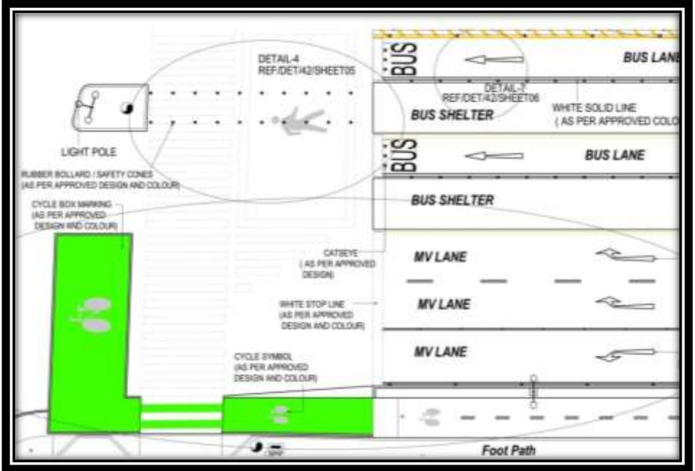
Figure 8-14: Typical marking at junctions for different road users
