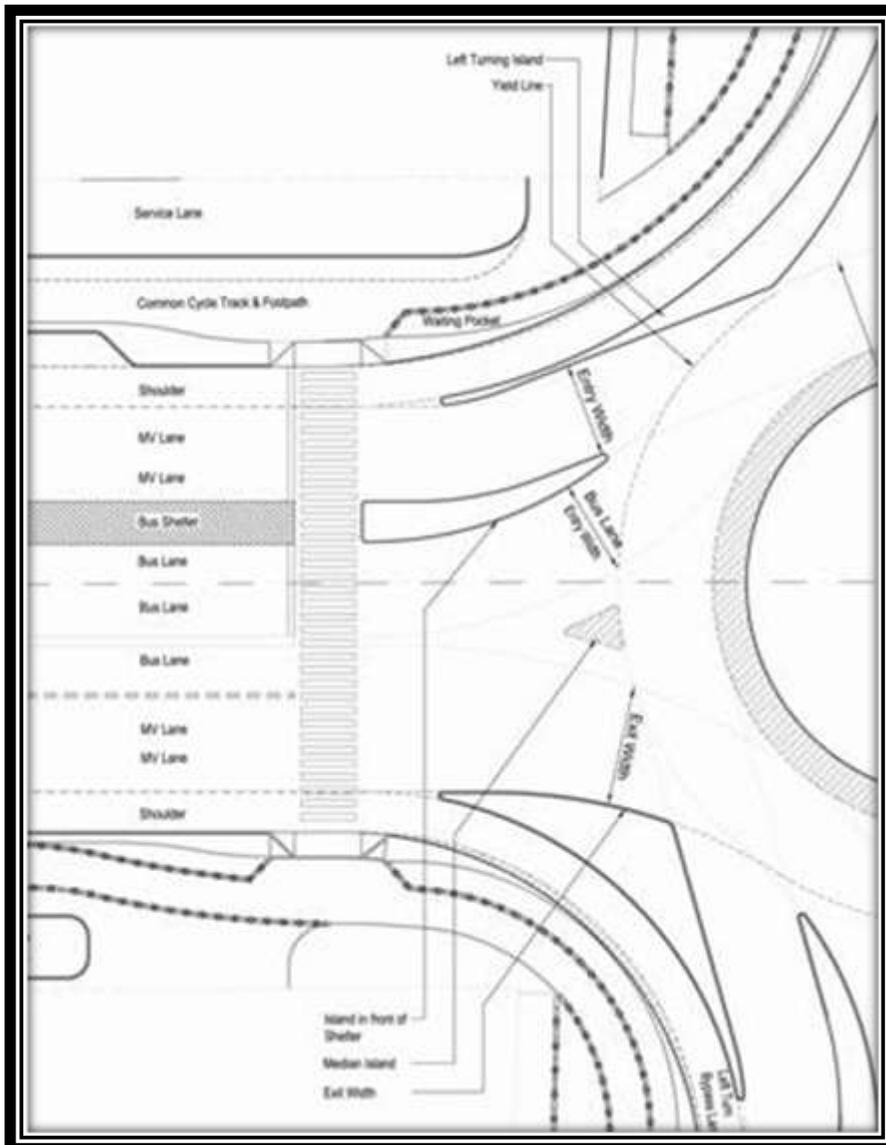
Figure 2-17 Various elements of a intersection
