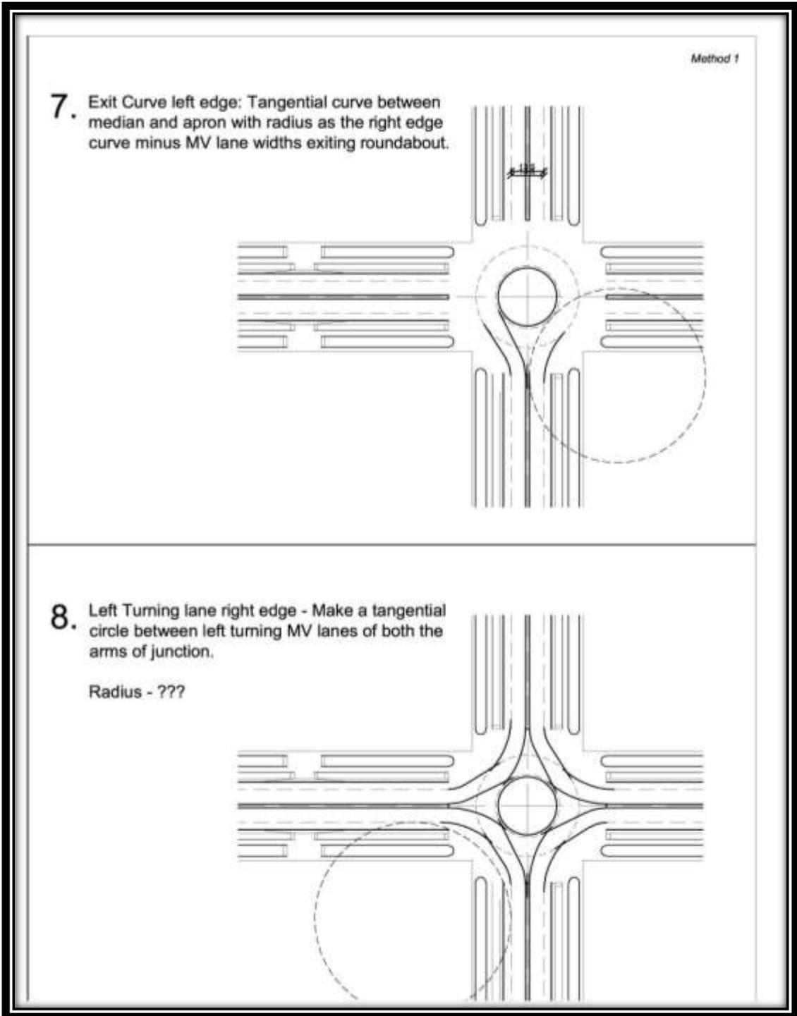
Figure 4-4 Tangential Method of Roundabout Designing (Step 7 & 8)
