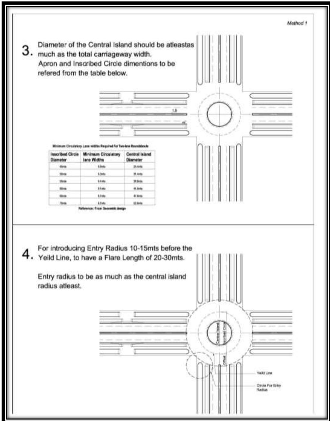
Figure 4-2 Tangential Method of Roundabout Designing (Step 3 & 4)
