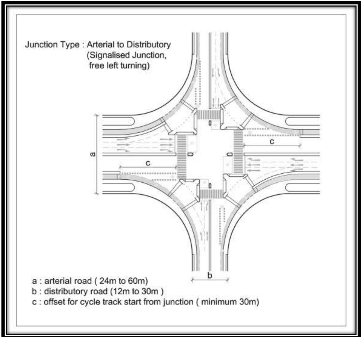
Figure 2-8 Signalized Intersection - Arterial to Distributor
