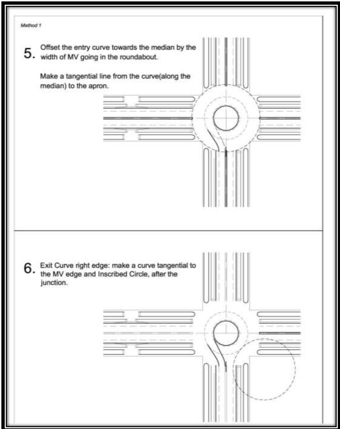
Figure 4-3 Tangential Method of Roundabout Designing (Step 5 &amp; 6)
