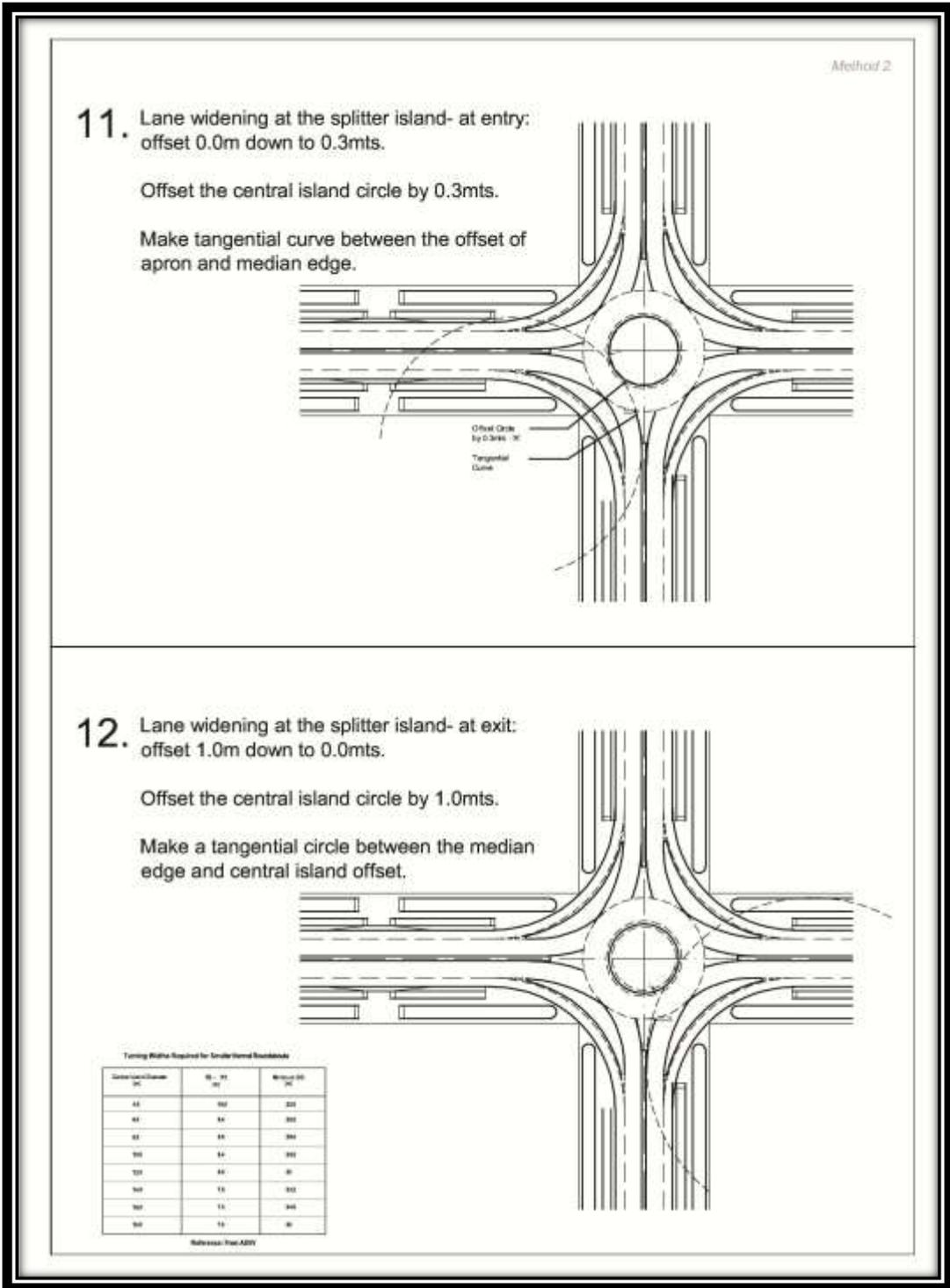
Figure 4-14 Lane widening at Splitter Island at circulatory roadway side Method of Roundabout Designing (Step 11 & 12)
