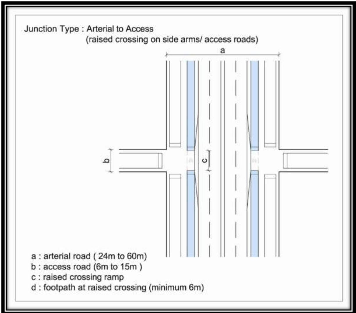
Figure 2-2 Arterial to Access – raised crossing on side arms
