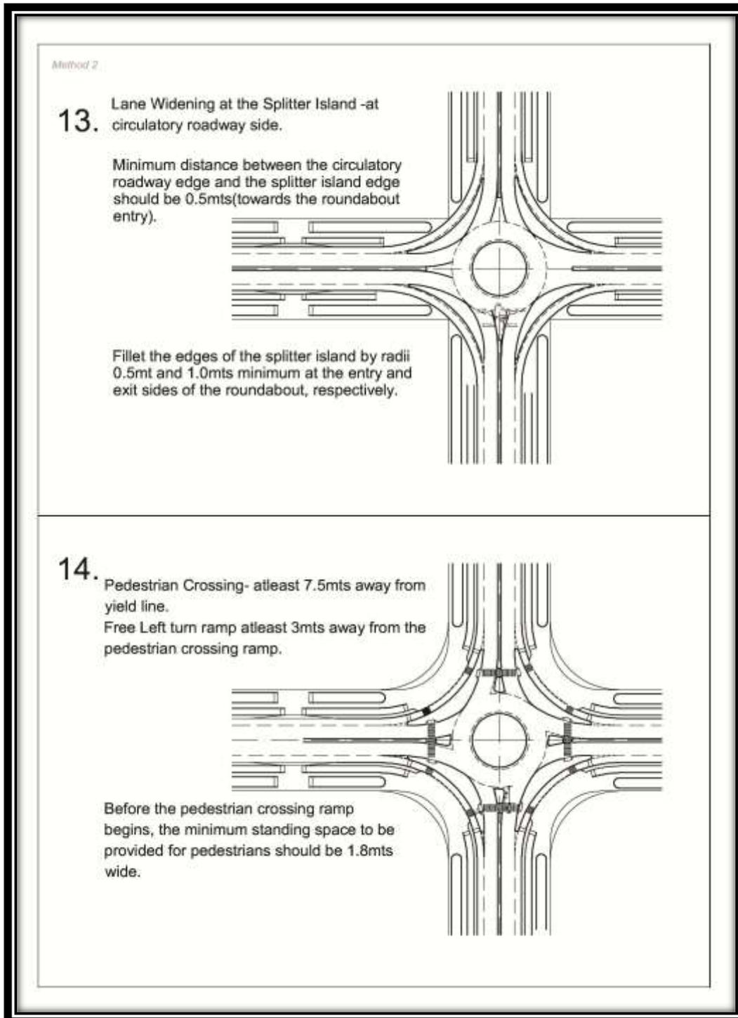
Figure 4-15 Lane widening at Splitter Island at circulatory roadway side Method of Roundabout Designing (Step 13 &amp; 14)
