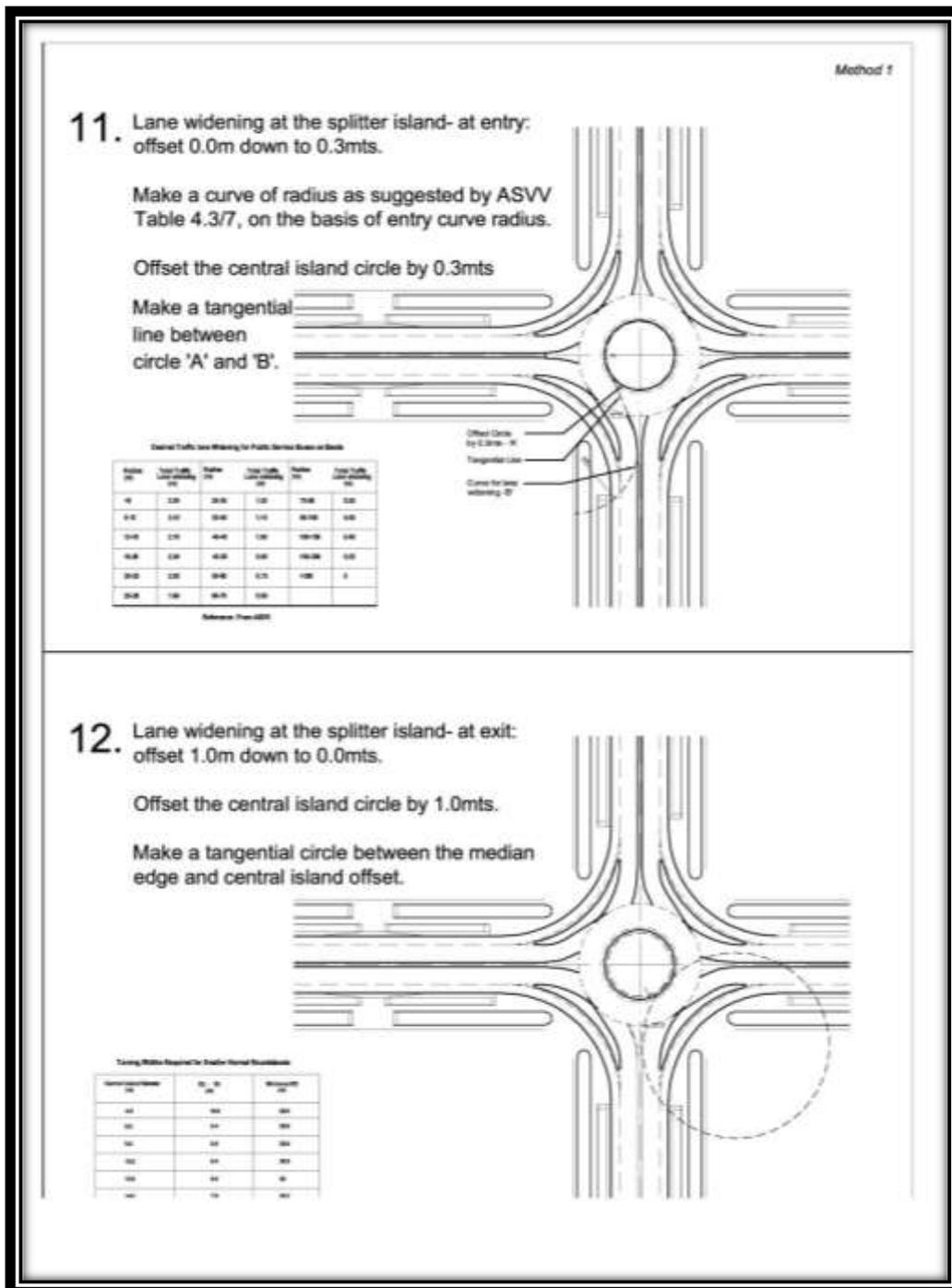
Figure 4-6 Tangential Method of Roundabout Designing (Step 11 & 12)
