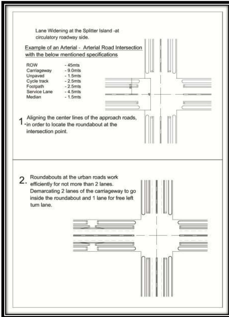
Figure 4-9 Lane widening at Splitter Island at circulatory roadway side Method of Roundabout Designing (Step 1 & 2)
