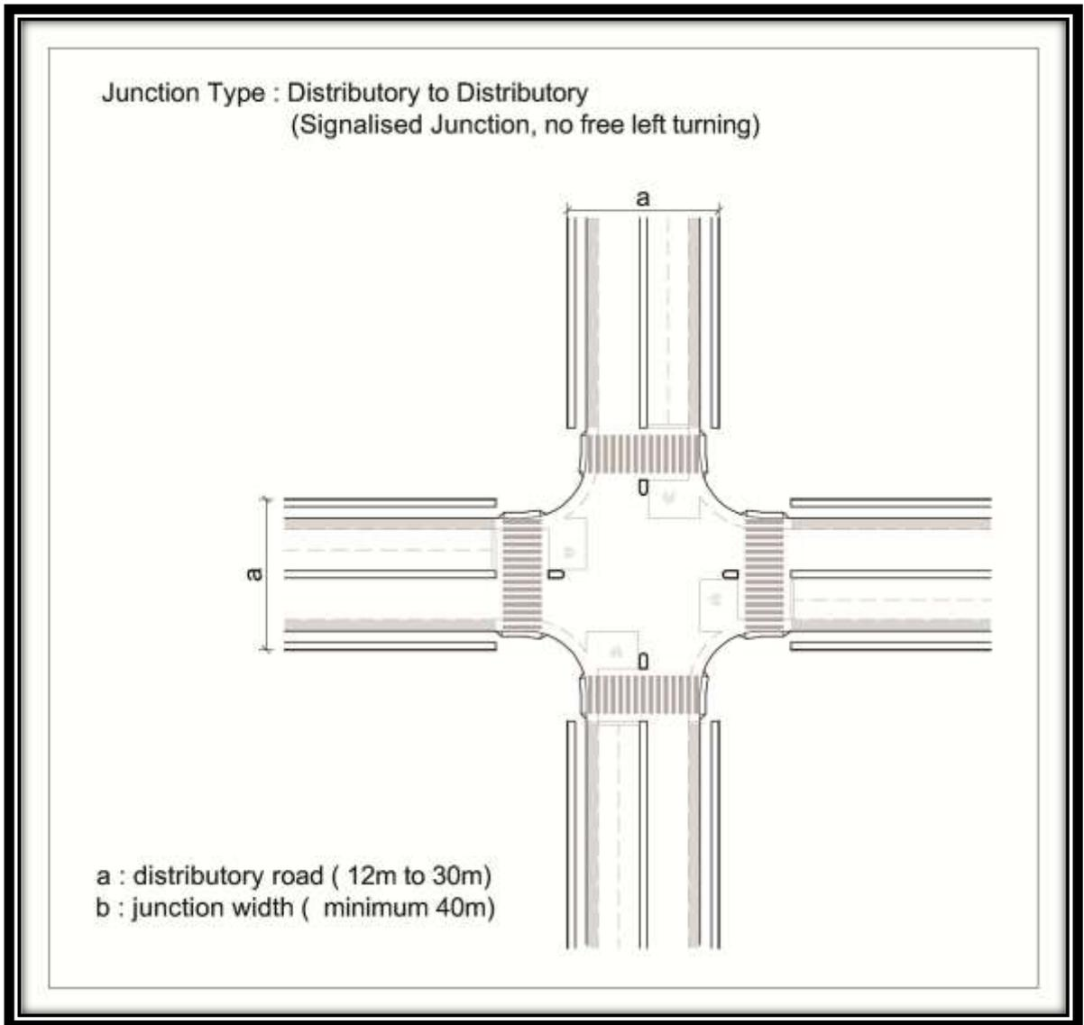
Figure 2-10 Signalized Junction - Distributor to Distributor
