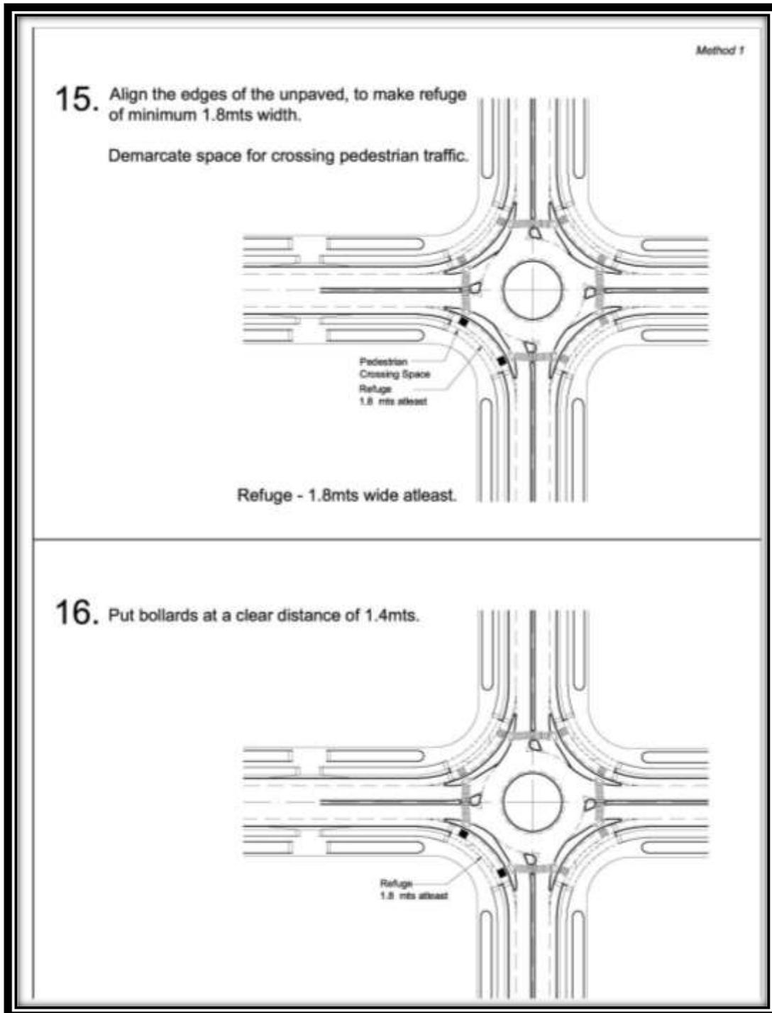
Figure 4-8 Tangential Method of Roundabout Designing (Step 15 & 16)
