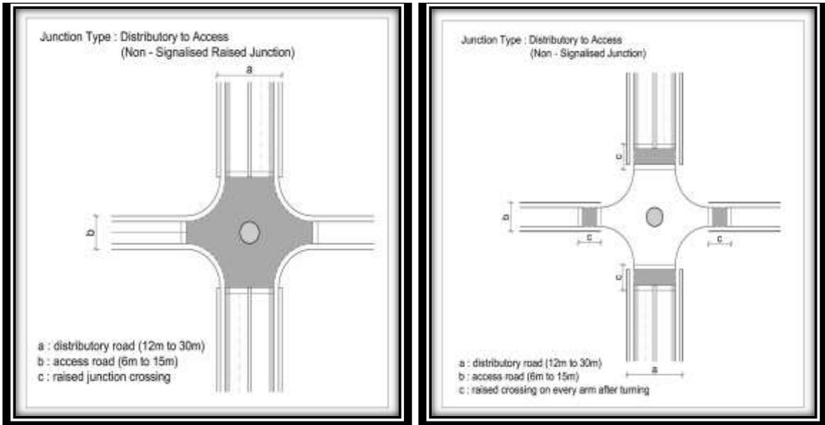
Figure 2-13 Mini Roundabouts (Distributory to Access)
