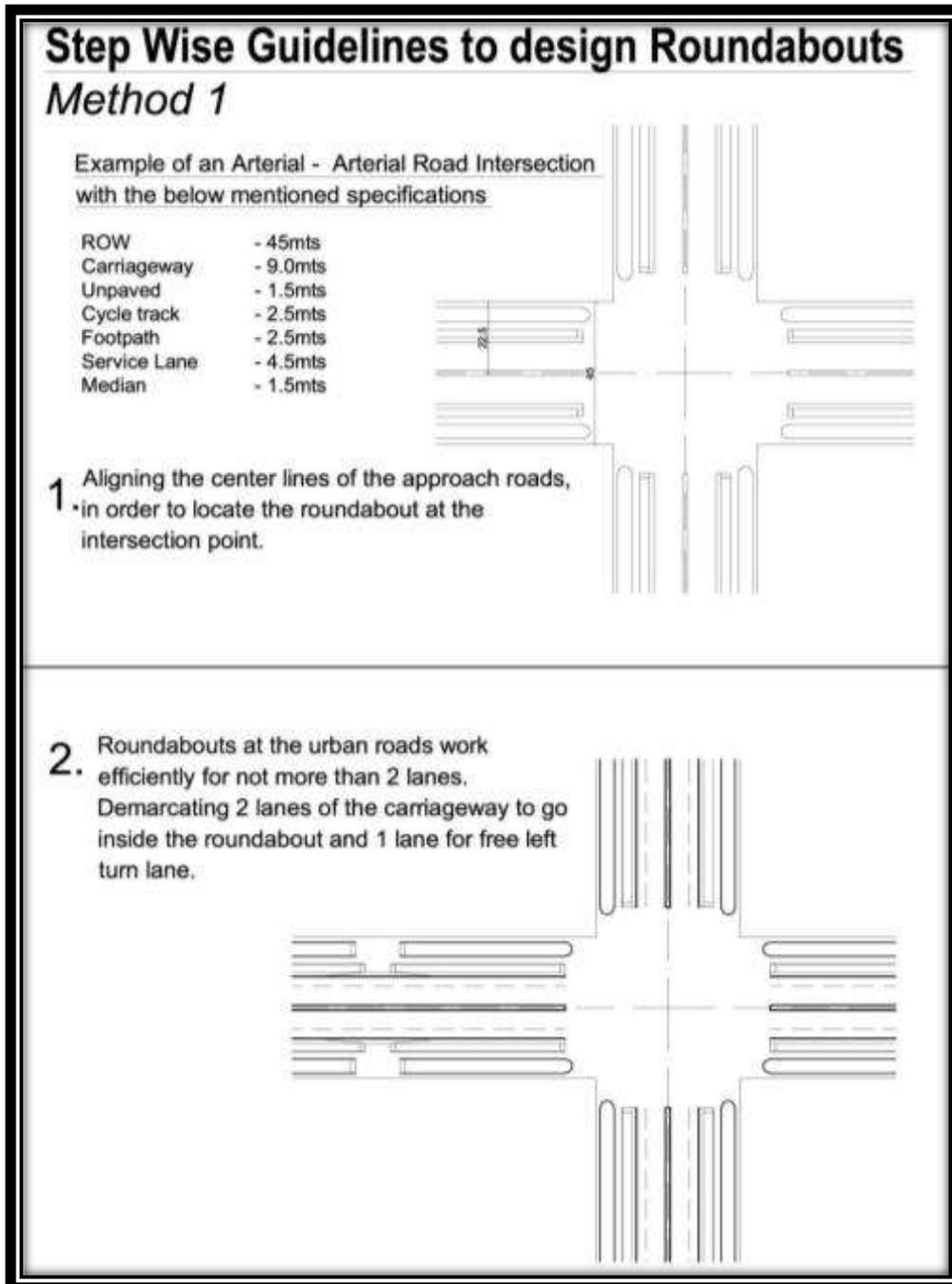
Figure 4-1 Tangential Method of Roundabout Designing (Step 1 &amp; 2)
