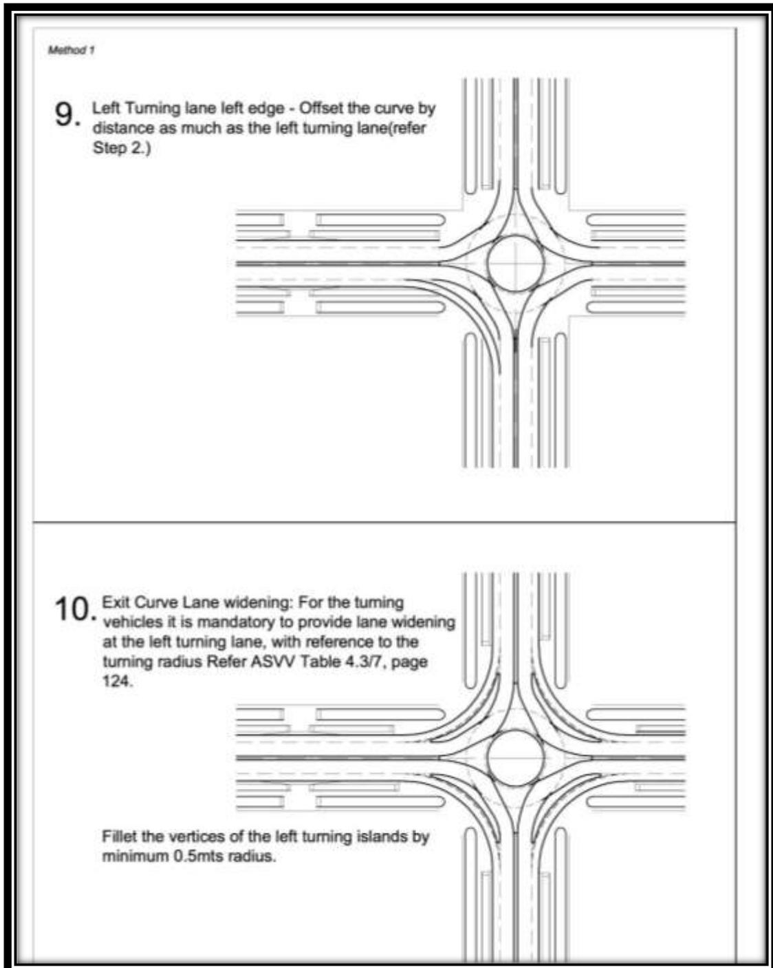
Figure 4-5 Tangential Method of Roundabout Designing (Step 9 &amp; 10)
