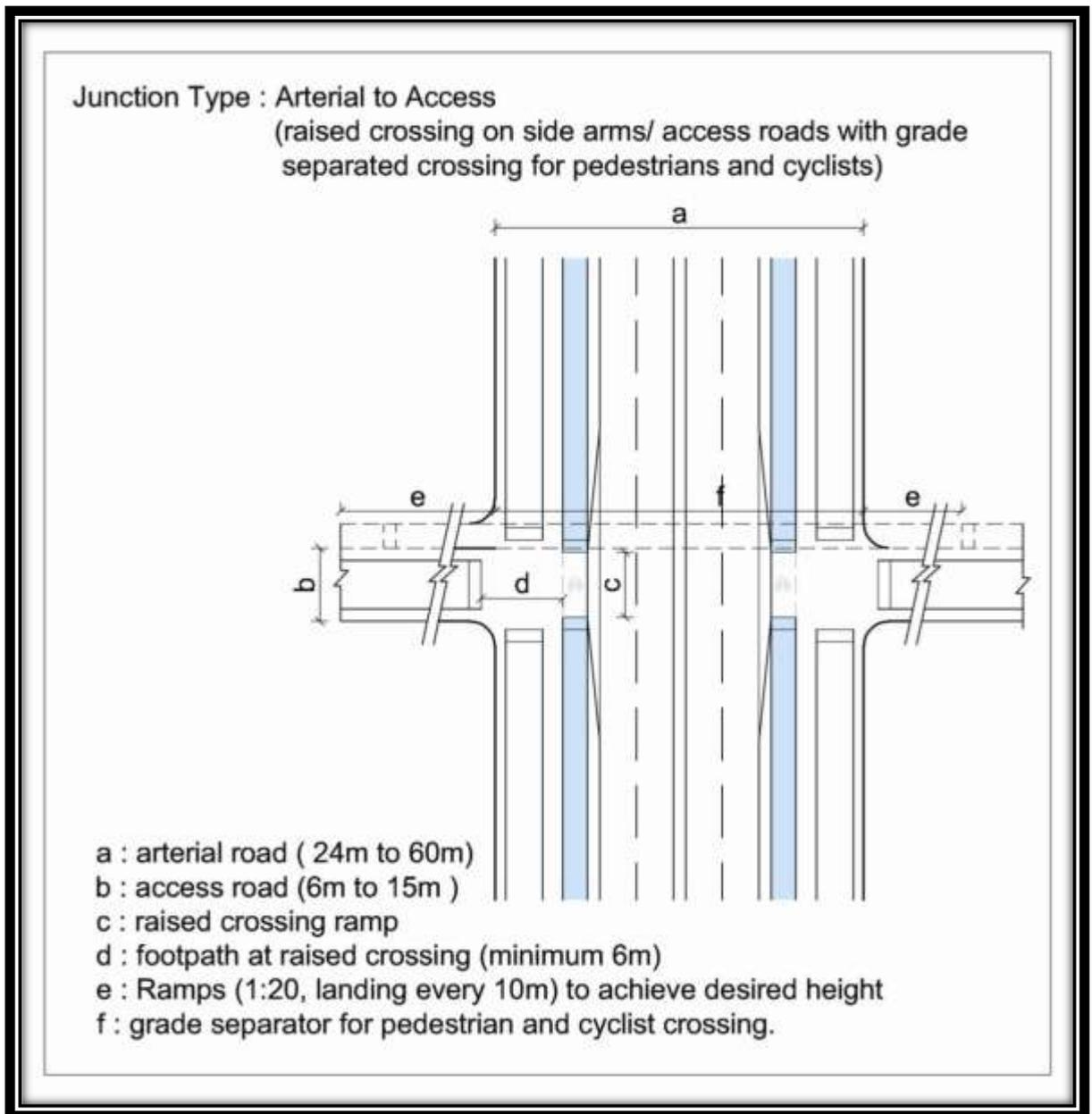
Figure 2-3 Arterial to Access – Raised Crossings on side arms with grade separated crossing for cyclists and pedestrians
