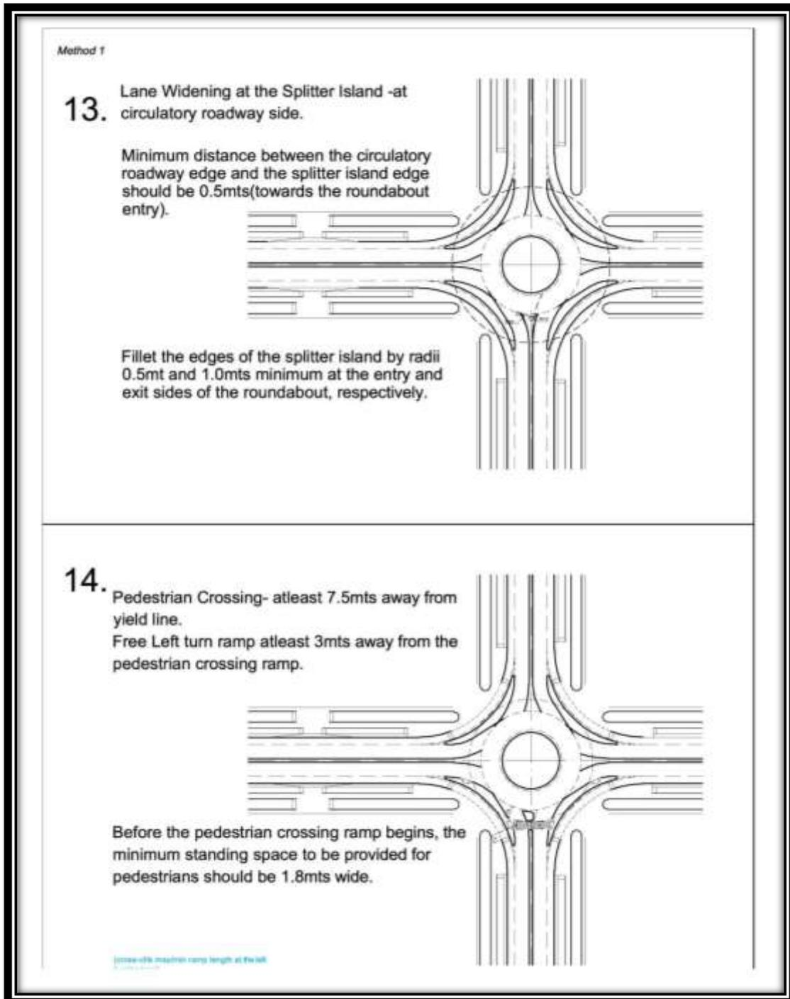
Figure 4-7 Tangential Method of Roundabout Designing (Step 13 &amp; 14)
