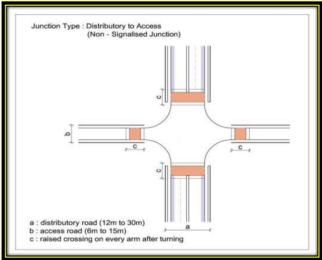
Figure 2-4 Non-Signalized Junction - Distributor to Access – raised crossings
